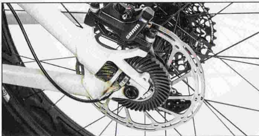
Here's the rear spiral bevel gears. Note the cable going in, which can connect/disconnect the AWD system via a lever on the handlebar.
