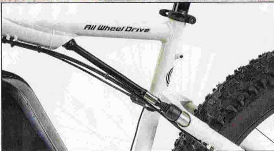
The rear drive shaft and universal joint are exposed on the left side.
